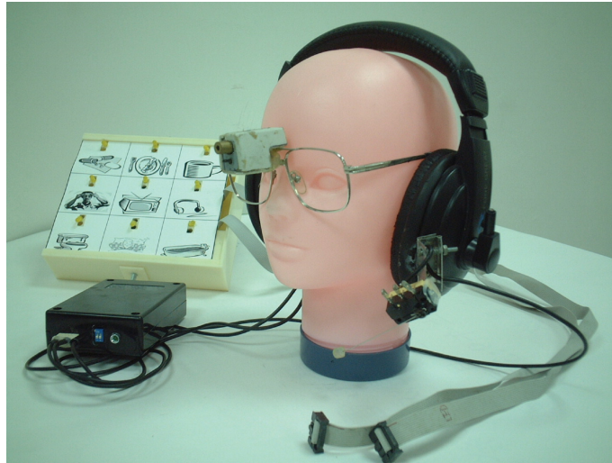
Figure 19: Infra-red home appliance control system
